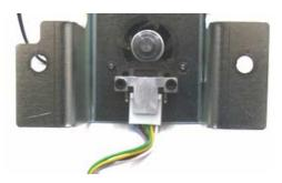
[3] Connect firmly the outer and middle coupling piece to the inner coupling (intact) while inserting the roller motor assembly.
