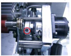
[10] Release the 2.5 mm coupling screw adjacent to the top back roller in order to adjust the coupling. Verify that all three couplings are secured together and there is no space between them. Once adjusted, secure the 2.5 mm coupling screw.
