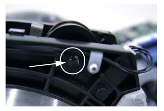
[6] Insert the flat screwdriver through the hole until it reaches the flat screw. Remove the flat screw securing the screen carriage to the plastic carriage holder.
