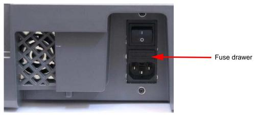
[4] Open the fuse drawer using a flat screwdriver to pull the plastic tab out gently from underneath.
