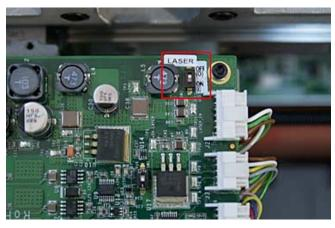
[2] Insert the safety interlock activation key into the safety interlock to the left of the roof assembly.
