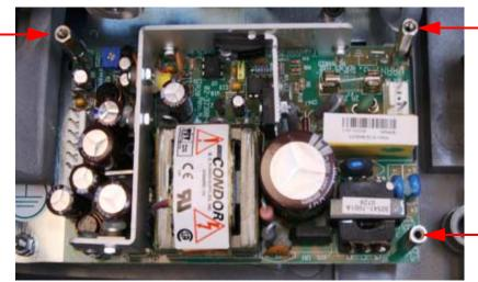
[9] Remove the power supply unit.
