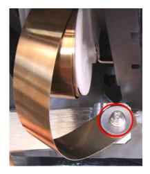
[5] Lift up the screen carriage until the screw is aligned with the small hole in the black plastic mold.
